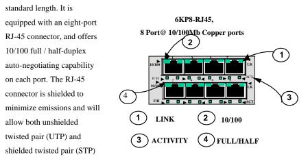
cable connections. The 6KP8-RJ45 module is equipped with a Media Dependent Auto-Crossover (MDI-X) switch, which controls all ports for cascaded connection. This feature eliminates the need for a special twisted pair crossover cable when connecting to a hub or another switch.
